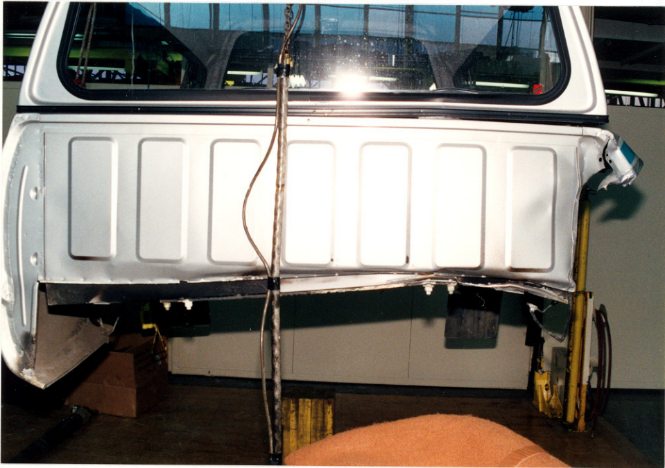
15. Frontal view of the cargo box and cap showing upward deformation along the left side from the CNG tank failure
